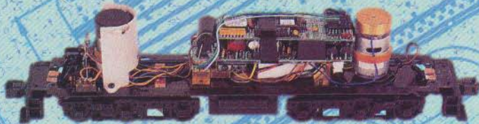
MTH and RailKing Locomotives feature a self-contained modular chassis for easy and quick servicing
